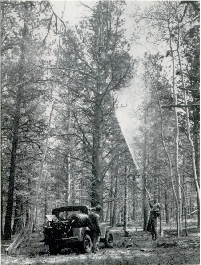
FIGURE 6.—One of the Jeep pressure-spray outfits and crew treating trees infested with bark beetles.
