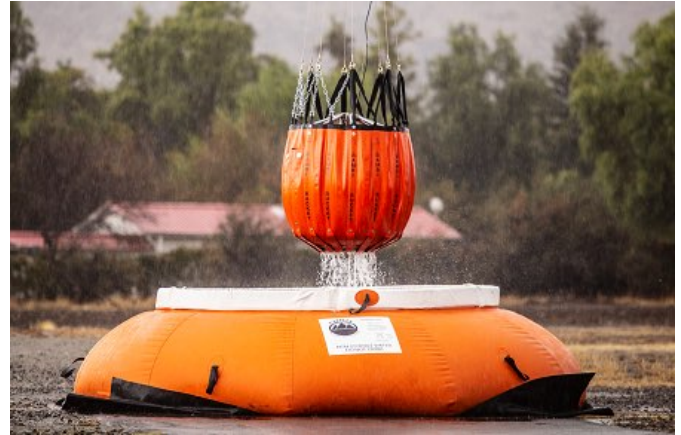
A Pumpkin Tank is the standard in helicopter bucketing operations. The Pumpkin Tank also serves as a portable water reservoir for fire departments and forest fire control agencies.
